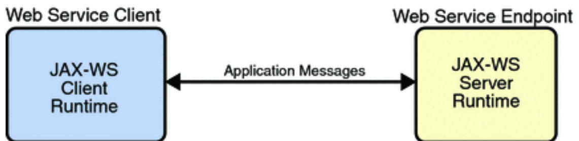
Figure 1.7. Application Message Exchange Without Reliable Messaging
